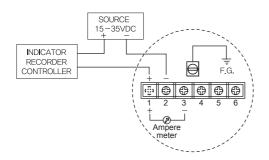
imesYou can check DC4-20mA output by connecting an ampere meter. (impedance: max. 30Ω)
